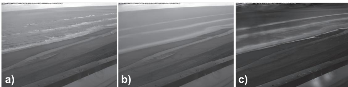
**Figure 1.2.** Example of the three types of images obtained from the Argus video system at Noordwijk station (6 February 2007): a) snap shot image, b) time-exposure image and c) variance image.
