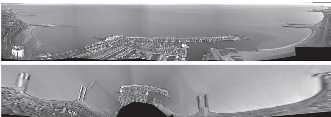
**Figure 1.3.** Example of the panoramic and rectified plan view obtained from the Argus station of Barcelona city beaches (21 October, 2001). Five individual time-exposure images are used to compose these merged images.
