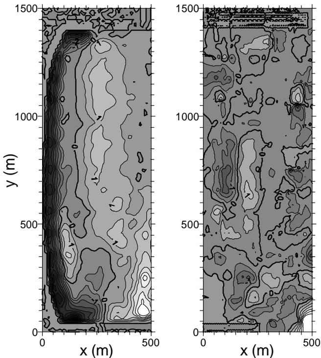
Figure 5. Differences in bed level between the final (November 3, 2003) and the initial (October 1, 2003) bathymetries. Dark colors mean erosion and light colors deposition. The zero contour line is indicated by a black thick line. Left: model. Right: observed.
