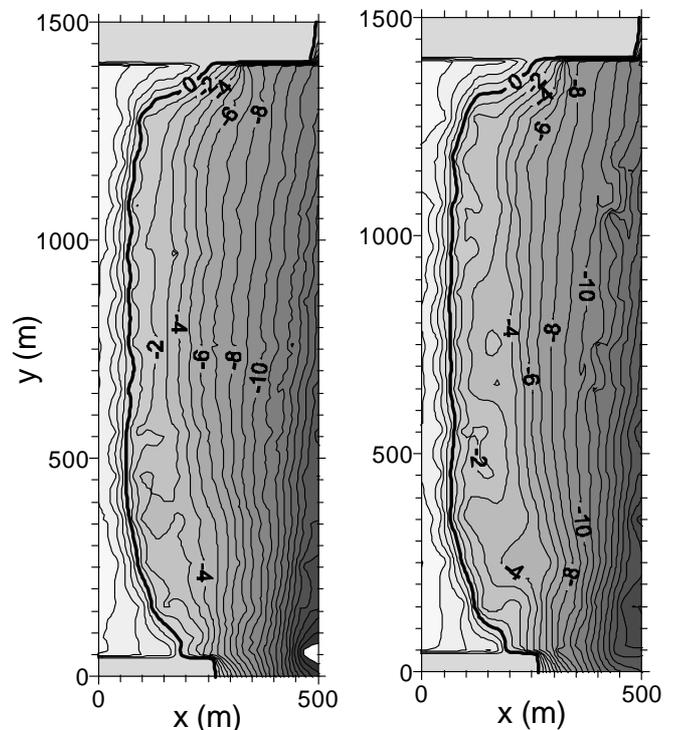
Figure 3. Surveyed bathymetry of La Barceloneta beach. The shoreline is indicated by a thicker line. Left: October 1, 2003. Right: November 3, 2003.
