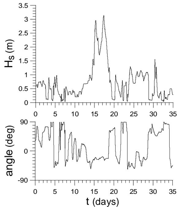
Figure 2. Significant wave height and wave angle at the offshore boundary of the model domain during the simulation period, from October 1 till November 4, 2003. The angles are with respect to shore normal ( $x$ -axis), positive from S, negative from E.
