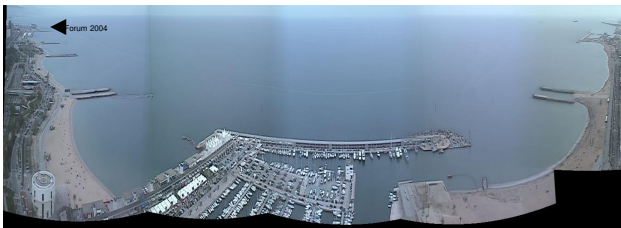
Figure 2. Merged Picture of Barcelona beaches and the Port Olympic. It corresponds to five images, each of them is the result of averaging out 600 images obtained during a 10 minutes sampling (1 image per second).
